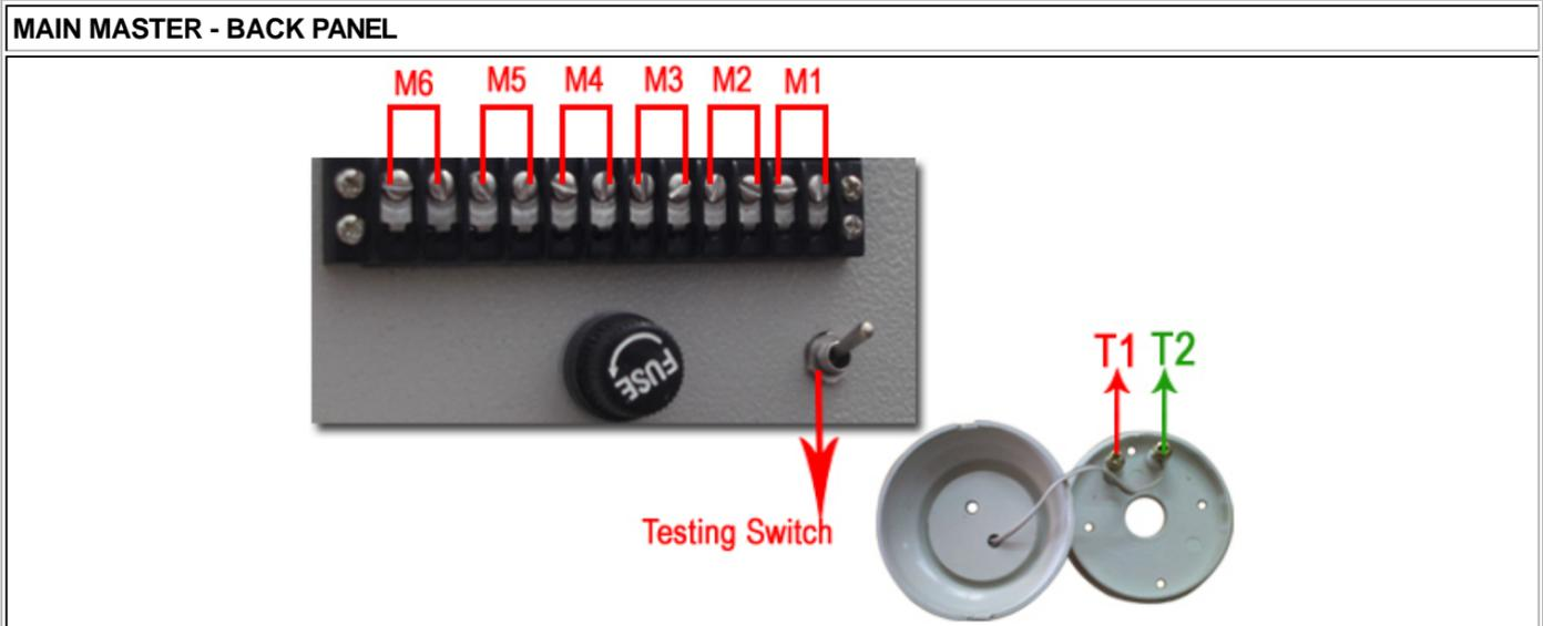
1. Connect first transducer **T1** & **T2** to the pair **M1** and place the Transducer beyond 10 feet (maximum 15 feet) from the Main Master console.
